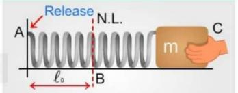
When point A is released then the spring force changes instantaneously to become zero.
