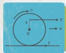
a = liner acceleration,  $\alpha$  = angular acceleration from linear motion
