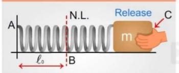
When the block is released at point C then spring force doesn't change instantaneously because of friction at mass m.
